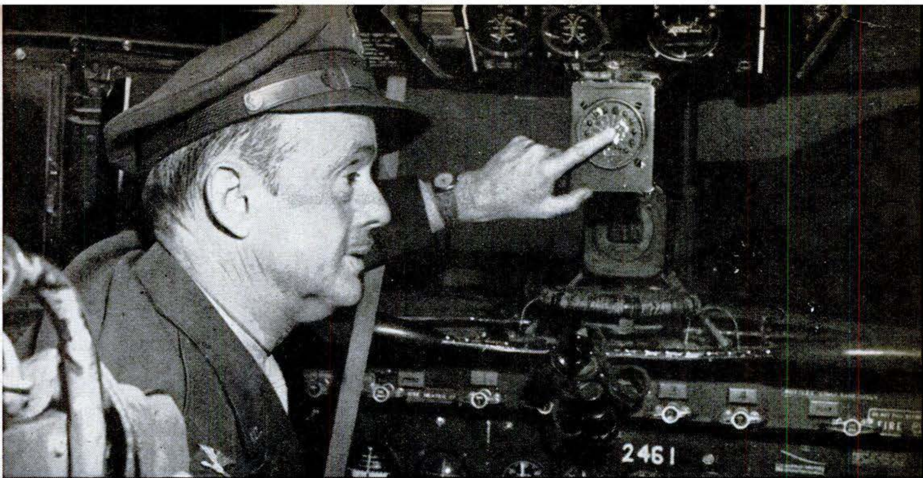
Colonel Gillespie points to push button that started Robert E. Lee on automatic flight.
